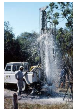
Resistivity surveying using an ABEM Terrameter (left), and test pumping borehole drilled by a Land Rover-mounted DHD rig (right).
