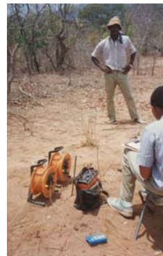
Resistivity surveying using an ABEM Terrameter (left), and test pumping borehole drilled by a Land Rover-mounted DHD rig (right).
